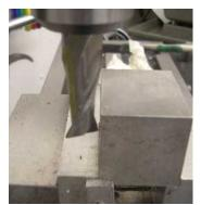
Since I will be cutting on the front side of the end mill, I push the 2 button. The end mill will barely scratch the back face of the block and the Y display will read 0.0000. If later I want to remove the offset, I just press the 5 button.
