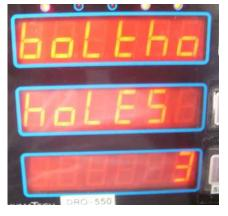
I chose 3. Sure hope I never need to enter 99! It could be handy if I was chain drilling a large hole. In fact, if you used a 2 flute end mill instead of a drill, you could us this function to rough cut a disk without using a rotary table.
