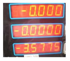
I then go to incremental mode and zero my X and Y axis. The function will use this incremental origin as the center of the bolt hole circle.
