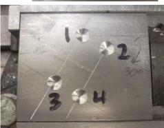
I have scribed lines between centers plus marked out the angle. Note that the 4 hole array has been rotated by 30 degrees. The holes are each 1/4" in diameter. The distance between holes 1 and 2 is 0.5". Between holes 1 and 3 is 1.0".
