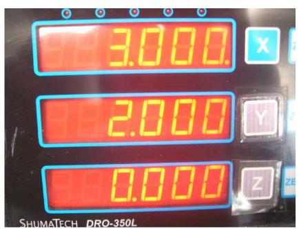
I have now cranked the X axis so my spud is 3.0005" to the right of my origin and my Y axis 2.0000". These are the exact value on the display. Please do not confuse the precision of the numbers with with the absolute accuracy of the DRO. That is a different can of worms<sup>3</sup>.
