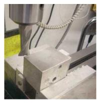
Say I have a block of metal and I want to cut a step on its back face. The back left corner of the block is at my absolute origin. I will use my brand new 5/8" end mill. Since it is new, I will assume it has a diameter of 0.625". It will be my tool number 2. On a critical job, I will later make a trial cut and verify that this assumption is correct.
