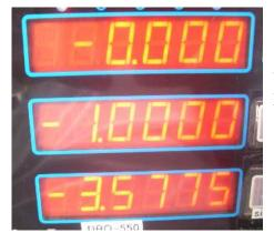
We are being told that the center of bolt hole 1 is zero inches along the X axis and -1.000 inches along the Y axis.
