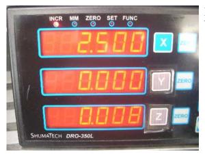
Say I want to move my Y axis INCR 0 such that I am at +0.5000". I first press the Y preset button and then input .5. the display shows 0.5" but internally it will be stored as 0.50000".
