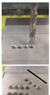
After drilling all 4 holes, you can see it came out fairly well. It doesn't take much time to get used to seeing a negative number show up on the X display and knowing that you must turn the crank in the positive direction to make it go to zero. Chain drilling goes very fast. Having the audible alert helps me to keep my eyes on the table motion until I get close to the next hole location.
