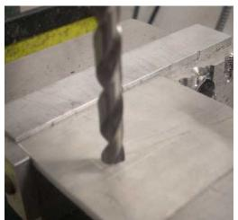
I scribed the front left corner of the slot and set my absolute zero there. Then I moved to (0.125, -0.125) so the drill is located at the start of the slot. I then changed to incremental and set my (0,0). Drill that first hole and push Enter.
