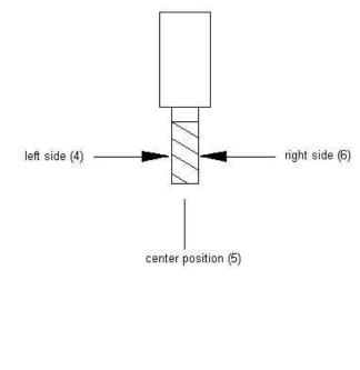
As viewed from the front of the mill, the end mill has a left side which is defined by pressing "4". The right side is selected by pressing "6". Press "5" to select the center position. The left and right side selections modify the X axis by adding or subtracting the end mill's radius from the displayed value. Front side is selected by pressing "2" and the back side is selected by pressing "8". The front and back sides modify the Y axis.
