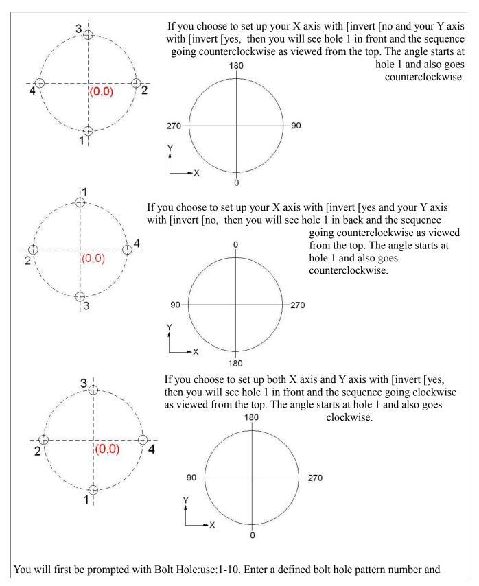
press Enter. You will then see a message saying which bolt hole is next. When you see the message, press any key to move to a numeric display showing you the distance to this hole. When you are done moving the mill table so the X and Y displays read zero, press Enter to move to the message related to the next bolt hole. You can only move forward through the holes. After the last coordinates are used, pressing Enter moves you to the message "Bolt Hole Done".
