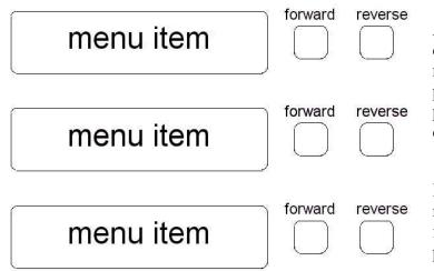
After Function has been pushed, the three displays take on new meanings. You navigate within a display by pushing the preset and zero buttons. In most cases, the preset moves you forward through the choices and zero moves you backwards.
