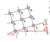
There is one more parameter that you must specify: the angle of the array. The array always pivots around hole 1 but the direction of rotation is a function of how you set up the axes as seen on page 28
