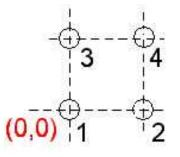
If you choose to set up both X and Y axes with [invert [no, then you will see hole 1 in the front left position with the angle set to zero.
