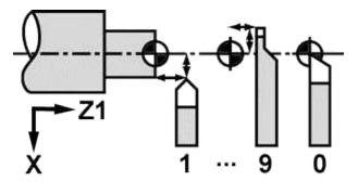
The first screen will prompt you to enter the tool offset number 1-16 with the numeric keypad. After pressing the number, you will be prompted to enter the X offset. When entering the offsets, press the
