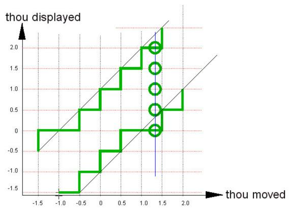
Again I have positioned the purple line relatively far from 0.0015" so it is clear which side of the transitions we are on.
