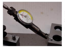
Stop for a moment and think about the repeatability and accuracy of a finger type Dial Test Indicator. Its value comes from being able to consistently tell you when the finger is in the same position relative to the indicator's body. This is an extremely useful thing to know in machining. The finger DTI has excellent repeatability, but its accuracy is limited. For more details, see <a href="http://rick.sparber.org/Articles/DTI/DTI.htm">http://rick.sparber.org/Articles/DTI/DTI.htm</a>.
