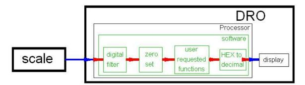
If we look at the hardware, we have between 1 and 3 scales connected to a box that I call the DRO. Inside the DRO are two key pieces of hardware: the processor and the display. The processor runs software.
