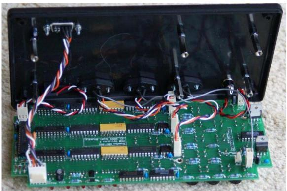
Note the gray wire going to the two pin header in the lower right hand corner. The gray wire connects to the ground wires of the scales.
