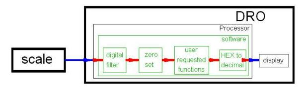
If things are very bad, we can have jitter on the scale's display. Most of the time we are talking about jitter on the DRO's display but here is where it can get confusing. Normally the HEX to decimal software is enabled so the
