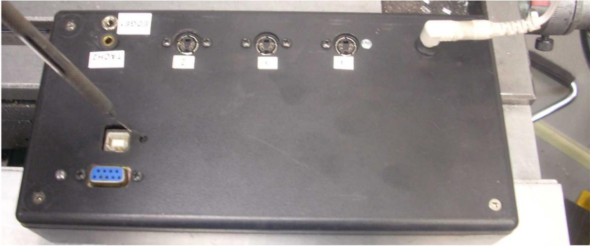
Here you see the USB connector peaking through the back of the DRO enclosure. The probe is pointing to the program pushbutton. You can also see my separate electronic edge finder and tachometer jacks in the upper left hand corner. I chose to not add connectors for Edge 2 or Flex 1 at this time. Flex 1 used to be called Tach 1.
