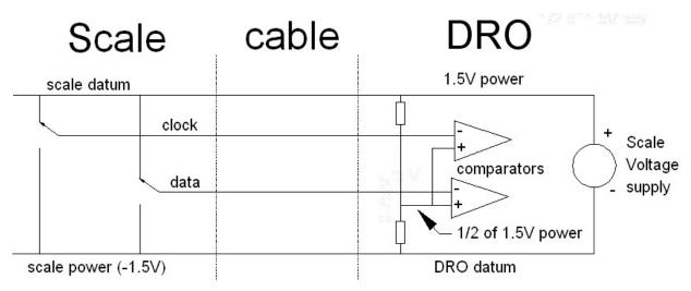
Now look at the clock and data switches and wires. The switches are actually in the electronics but showing plain switches does not diminish the accuracy in any significant way. These switches move up and down as pulses are generated. In the up position, these signal leads are connected to scale datum. In the down position, they connect to scale power.
