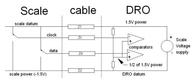
Note the boxes labeled Z1, Zc, Zd, and Z2. If we are concerned with just direct current, then Z represents a resistance. If we are concerned with AC, then Z represents a resistor with an inductor in series. This means that as the frequency of the noise increases, the "impedance" gets larger. The larger the impedance, the easier it may be to get noise into our comparators. If all 4 conductors are in the same cable, all Zs shown here are equal.
