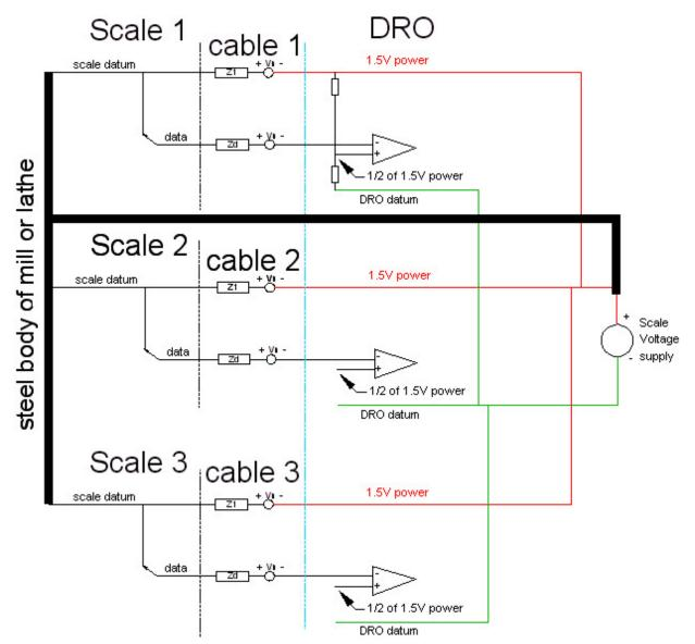
This will force the voltage on the scale datums to be the same as at the Scale Voltage supply's positive net. Any noise associated with Z1 in any cable will have no effect on the scale datum. You will still have to contend with the noise associated with the data lead. Noise from other cables will not effect this cable.
