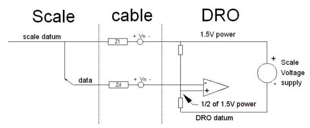
I hope you can still see that the voltage seen at the negative input of the comparator is immune to the noise voltage Vn.
