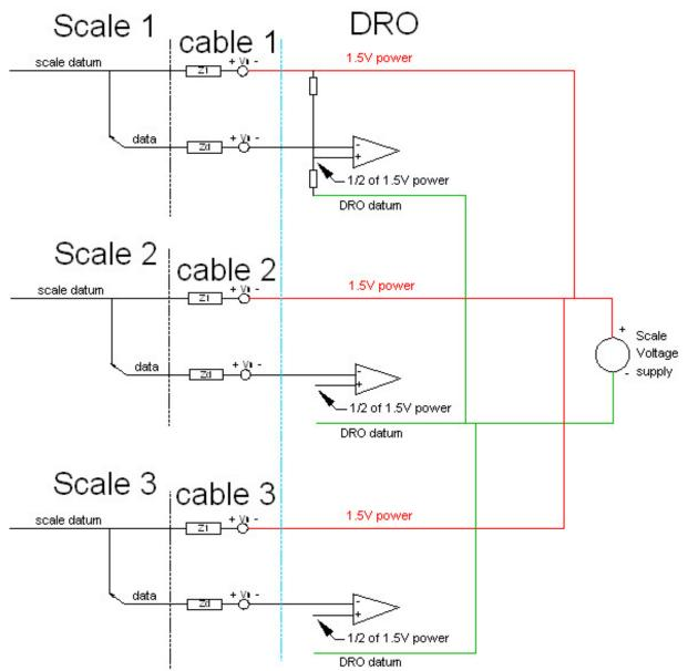
Each cable can be a different length and have a different exposure to noise. This means that cable 1's Z1 and Vn may not be the same as cable 3's Z1 and Vn. It turns out that this does not matter. The noise associated with each cable is canceled as seen by the associated comparators as explained above. So having three independent scales is no different from having just one.
