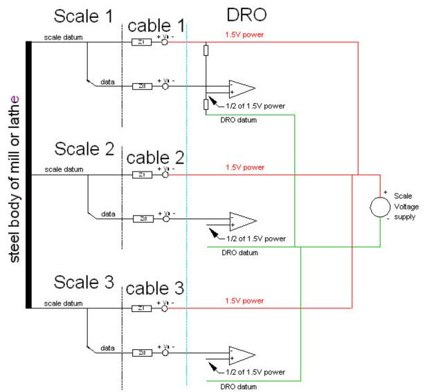
Making the electrical connection from each scale body to the steel of the machine greatly complicates how the system responds to noise but that does not mean it is a bad choice. I have all of my scales connect this way on my mill and it works fine. I have also heard of people who do not connect their scale bodies this way and who have seen problems. It all depends on how much noise your system must tolerate.
