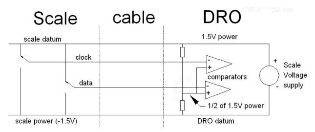
The first point of confusion is how things are named. Documentation related to the connections on the scale talk about +1.5V, ground, clock, and data. The +1.5V connection is also connected to the metal on the scale. It is standard practice to make the metal body associated with an electronics package the ground. Now, ground is a confusing term. In any system, you are free to define any single point as "ground". Ground is the reference point that is used to measure the relative
