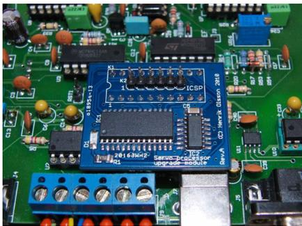
Module mounted on HP-UHU
