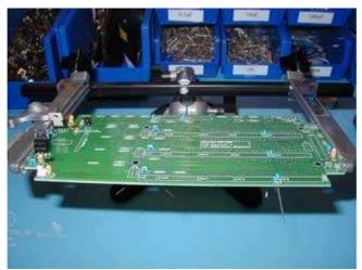
Step 3. Install the Decoupling Capacitors
