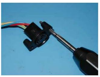
Tap the Mini-Din Scale Connectors with an M2.5
