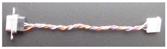
Programming Cable DB-9 Serial Connectors
