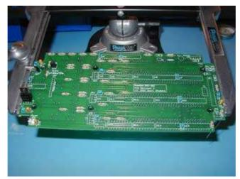
Next, install all of the resistors. It is easiest to use a triangular <u>lead forming tool</u> but not required. The resistor lead are spaced at 400 mil. Run through the BOM installing each resistor value at its correct designator. It is easiest to solder the resistors from the component side. After soldering, you probably want to run back through the BOM double checking the correct resistor values.
