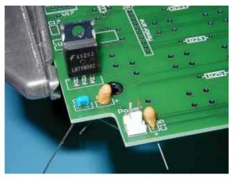
The 5 volt power supply consists of device U16 and capacitors C3, C4, and C15. An optional MTA-100 connector can also be used for the power entry connector JP6. Pay special attention paid to the polarity of C15 and C3. These are tantalum capacitors and have a marking on the POSITIVE lead. Make sure to insert the marked lead to the side marked with a + on the PCB. Also notice that the pad this lead is inserted into is square instead of round.
