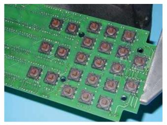
Install the seven tact switches on the <u>display</u> side of the PCB from the components. There is nothing special to installing the tact switches other than to make sure they are fully seated in the PCB. Flip the PCB over and solder all of the tact switch leads from the component side of the PCB.
