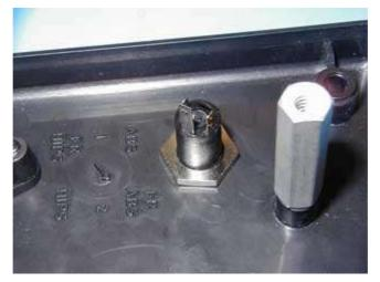
Auxiliary Connector Mounted to the Back Panel with the Included Nut (Replace with UK picture when available)
