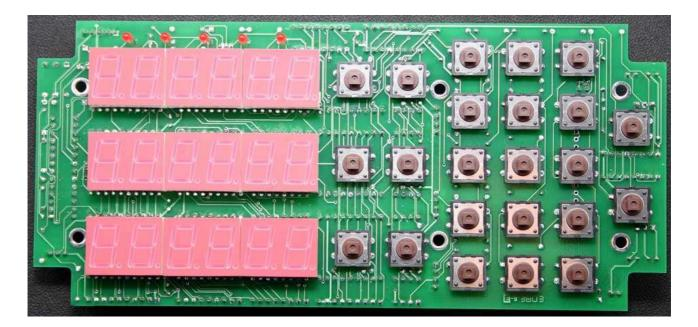
Display Side of a Completed DRO-350 PCB
