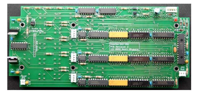
Component Side of a Completed DRO-350 PCB
