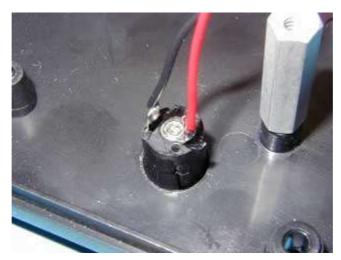
DC Power Connector Pushed Through the Hole in the Back Panel (Replace with UK picture when available)
