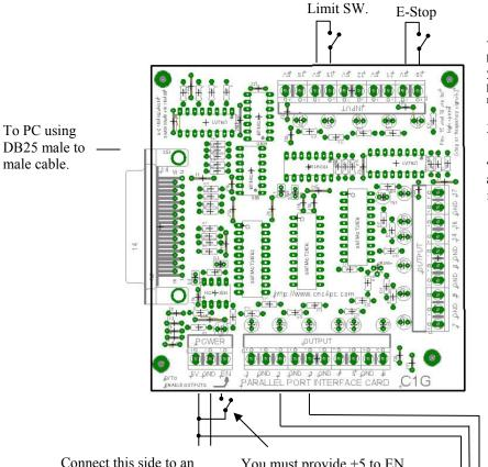
Connect this side to an external +5vdc power supply to power your card.
