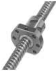
TYPE: DINF DIN69051 Class 7 Backlash (0.052um/300mm)
