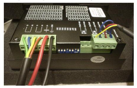
The stepper cable from the motor then goes red to A, yellow to A1, blue to B and green to B1 This applies to all three drives. The two terminals marked Enable are not connected. IT IS IMPERATIVE THAT THIS WIRING IS KEPT TO AND DOUBLE CHECKED.
