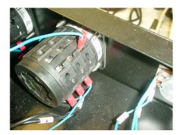
Remove the three cables from the speed control potentiometer at the speed board end marked P1, P2 and P3,
