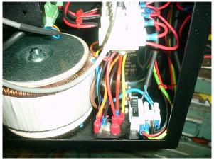
This completes the power side of the installation and if a temporary mains feed is fed to the mains fuse holder and the 7 amp mains fuse is fitted you should have about 63 to 65 volts DC across the stepper fuse holders.
