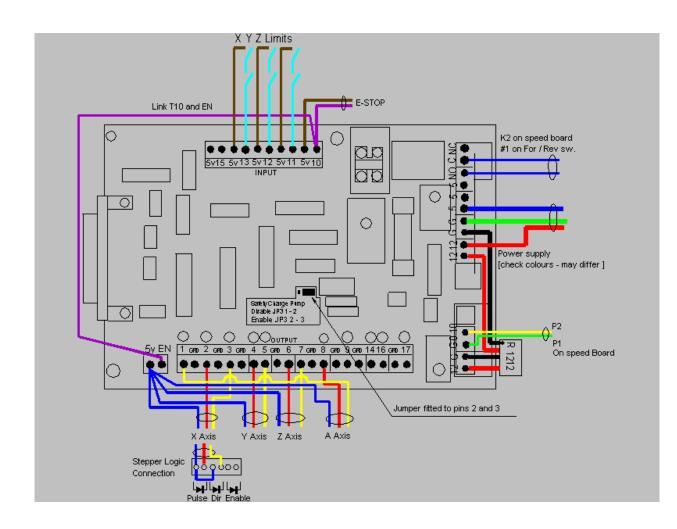
The logic to the stepper drives is carried by three [or four] separate light 4 core cabling. Use blue for 5v, red for step and yellow for direction, green is cut back.
