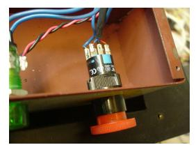
We need to use two terminals that are broken when the switch is pressed. Using the multimeter set to continuity and with one end pin as common find which of the other two pins is broken when the E-stop is pressed. The usual layout is how the other set of terminals are used but double check with a meter. Using the length of twin cable supplied solder a wire to each and thread this cable back through the conduit to exit out the lower panel access.
