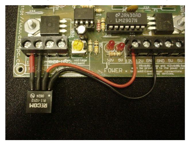
On the right hand side of the board the connections are ground on the power supply to ground, 5 volts to 5 volts, 12 volts to 12 volts.
