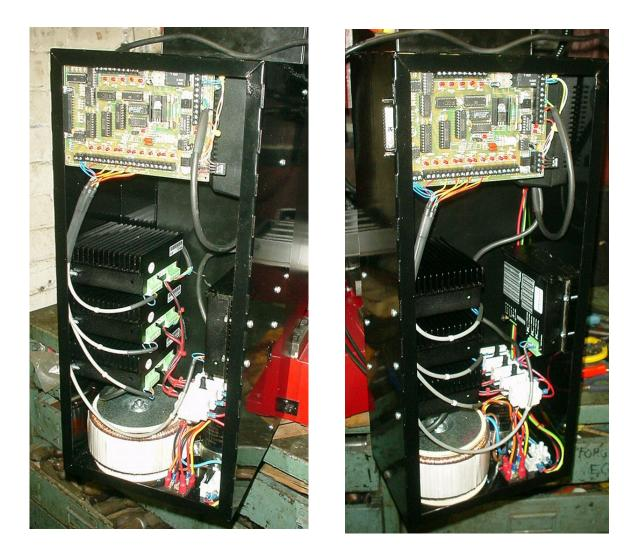
On the output side of the mains fuse holder the brown transformer cable goes to the fused side and the blue cable goes to the opposite end. The centre connection is left empty at this stage for the earth cable when the enclosure is fitted.
