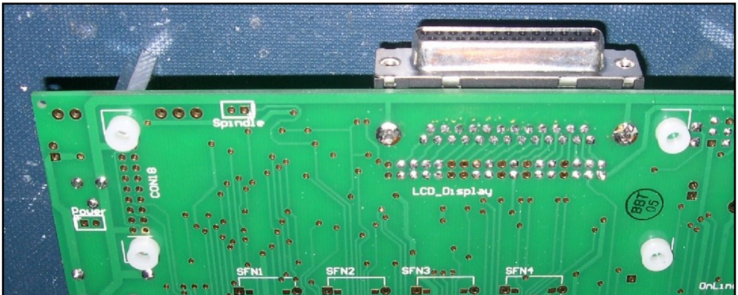
Figure 7b. Spacers placed where LCD is to be installed.
