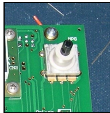
Figure 11b. Installed MPG
